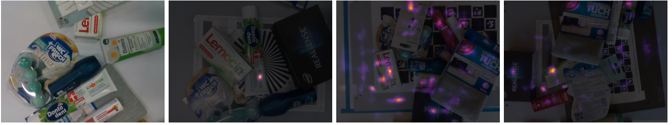
Fig. 2: Visualization of the matching uncertainty. The red circle in the left most image marks the sampled keypoint. The following test images are superimposed with the predicted distribution as heatmap. If a correspondence exists (second from left), the mass of the distribution is well localized. If no correspondence exists (middle right and right most image), the mass is spread over various areas that are the most similar in descriptor space. Viewed best in color.
