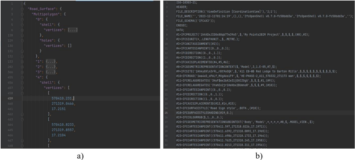
Figure 11. Different data storage strategies: a) geometric information stored in JSON and b) 3D gDTs stored in IFC.
