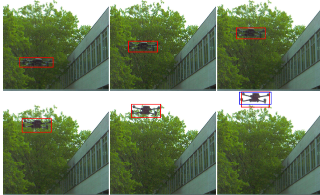
Fig. 1. Visual comparison between YOLO-FEDER FusionNet (red bounding boxes) and YOLOv5l (blue bounding box), showcasing every fifth image frame. YOLO-FEDER FusionNet consistently detects the drone across all six frames, whereas YOLOv5l only identifies it in the last one.
