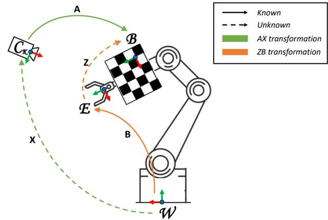
Fig. 2. Single-camera hand-eye calibration setup, used to derive the homogeneous transformations  $AX = ZB$ . Here,  $A$  denotes the camera-to-board transformation and  $B$  represents the pose of the robot’s end-effector relative to its base  $W$ . While  $X$  and  $Z$  are the two unknown transformations.
