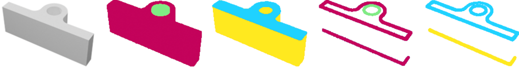
Figure 1: Example of segmentation prediction. From left to right: input rendered image, surface instance segmentation, surface start-end-barrel segmentation, curve instance segmentation, and curve start-end segmentation.
