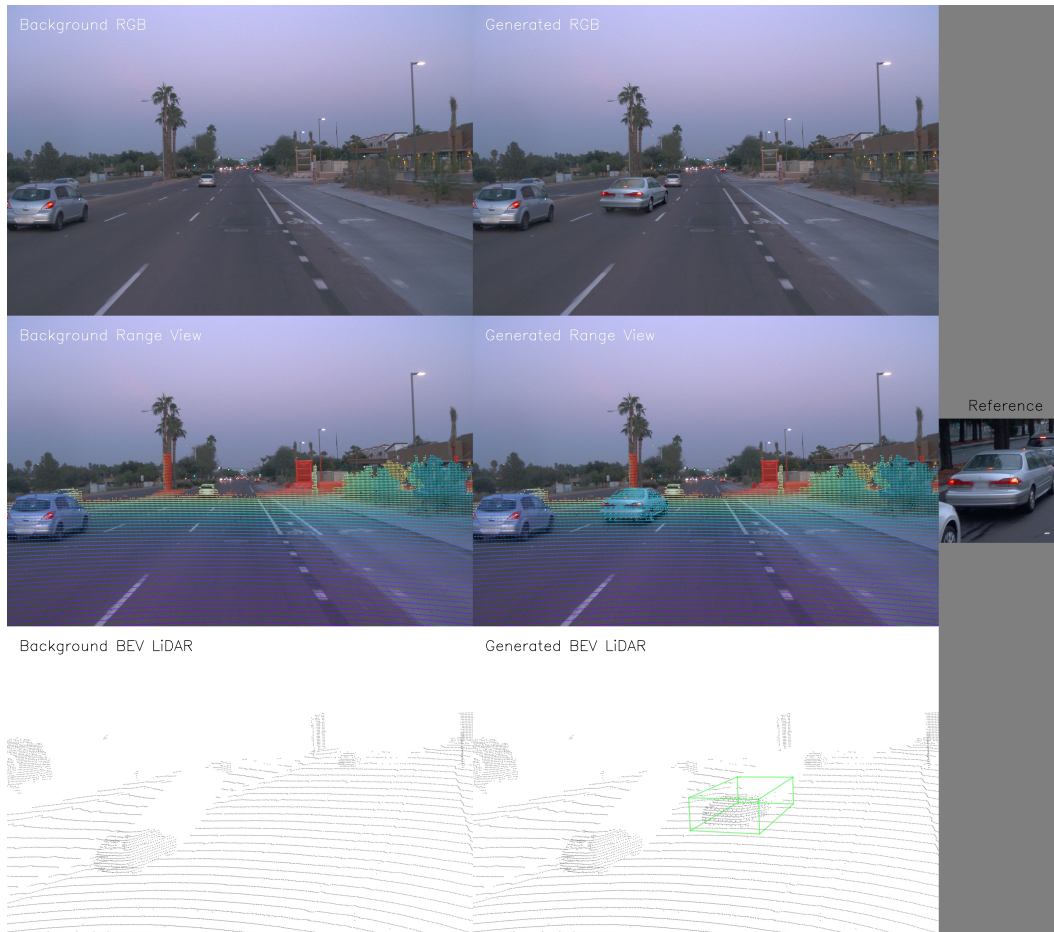
Figure 12: Multi-modal Video object insertion. Left: input frame, Middle: generated frame, Right: reference car. We insert a back view of a car and show its corresponding LiDAR map. The middle row highlights that our image and LiDAR point clouds are aligned after synthesis.
