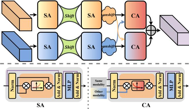
Figure 4: The cross-attention mechanism architecture. ‘‘SA’’ follows the standard transformer architecture which contains one self-attention block. The ‘‘Shift’’ and ‘‘unshift’’ mean the block shift and shift back operation. ‘‘CA’’ indicates the novel cross-attention mechanism which focuses on the uncorrelation information.
