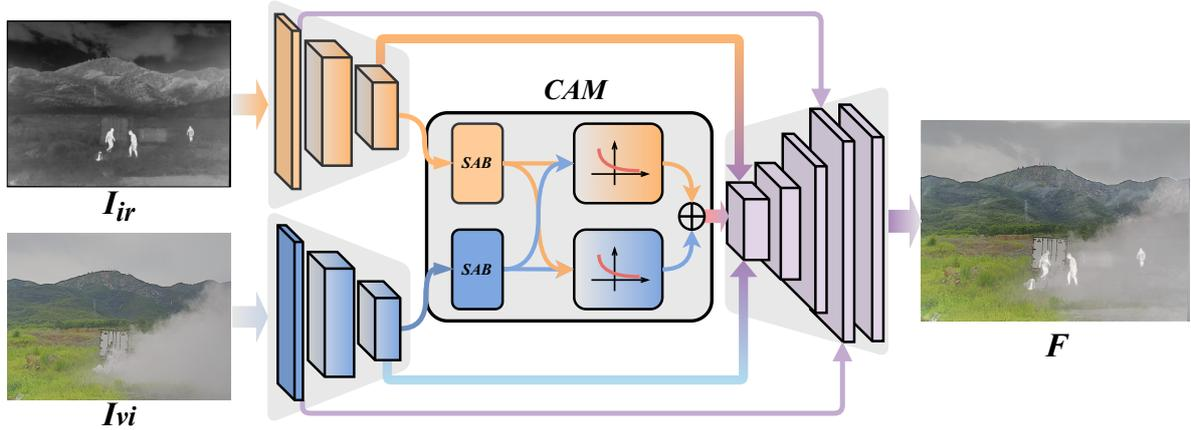
Figure 2: The framework of CrossFuse. Two “Encoder” contain same architecture but different parameters. The cross-attention mechanism (CAM) is utilized to fuse the multimodal features. “SAB” indicates the self-attention block. The fused image can be obtained by “Decoder” with the long connection from encoders.
