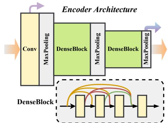
Figure 3: The encoder architecture which contains three blocks: “Conv”, “MaxPooling” and “DenseBlock”. “Conv” indicates one convolutional layer, “DenseBlock” includes four convolutional layers with dense connection.
