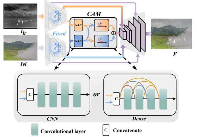
Figure 11: The proposed network with different fusion module: CAM, CNN and Dense.
