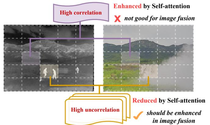
Figure 1: The correlation and uncorrelation for self-attention in image fusion task. For multimodal images, the self-attention may not be suitable for inter-modality processing. In image fusion task, the redundant information will be enhanced and the complementary features are reduced, which is more obvious when the source images are all in gray-scale.
