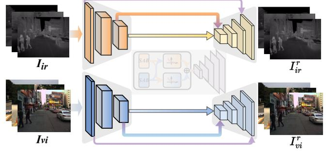
Figure 7: The first training strategy. Two auto-encoders are trained to reconstruct the inputs (infrared images and visible images).
