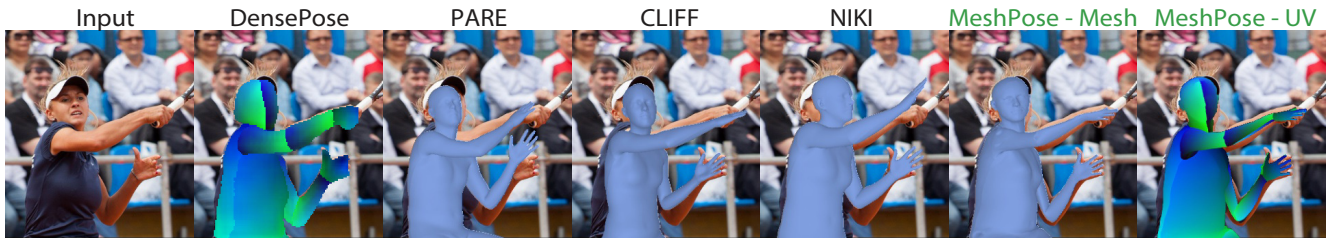
Figure 1. DensePose prediction systems are pixel-accurate but do not provide a 3D mesh, while human mesh recovery systems do not provide pixel-accurate 2D reprojection. We propose MeshPose, a novel human mesh recovery method that combines the benefits of both.
