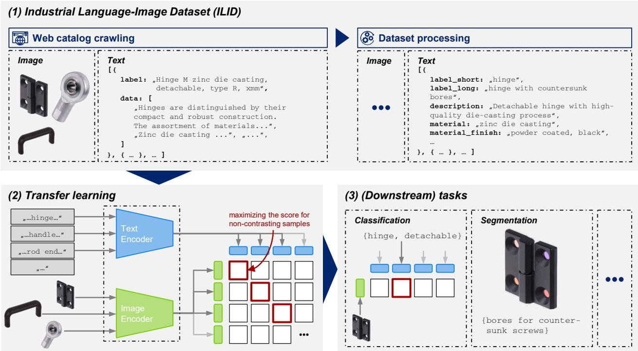
Figure 2. Overview of this work’s method: (1) generation of the Industrial Language-Image Dataset (ILID), (2) transfer learning using the ILID, and (3) evaluating the performance in different tasks.
