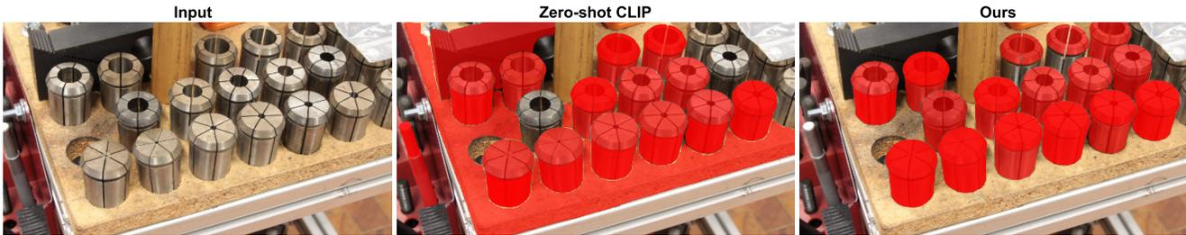
Figure 10. Language-guided segmentation results given prompt "collet" compared to zero-shot CLIP under the same settings (segmentation properties and thresholds).
