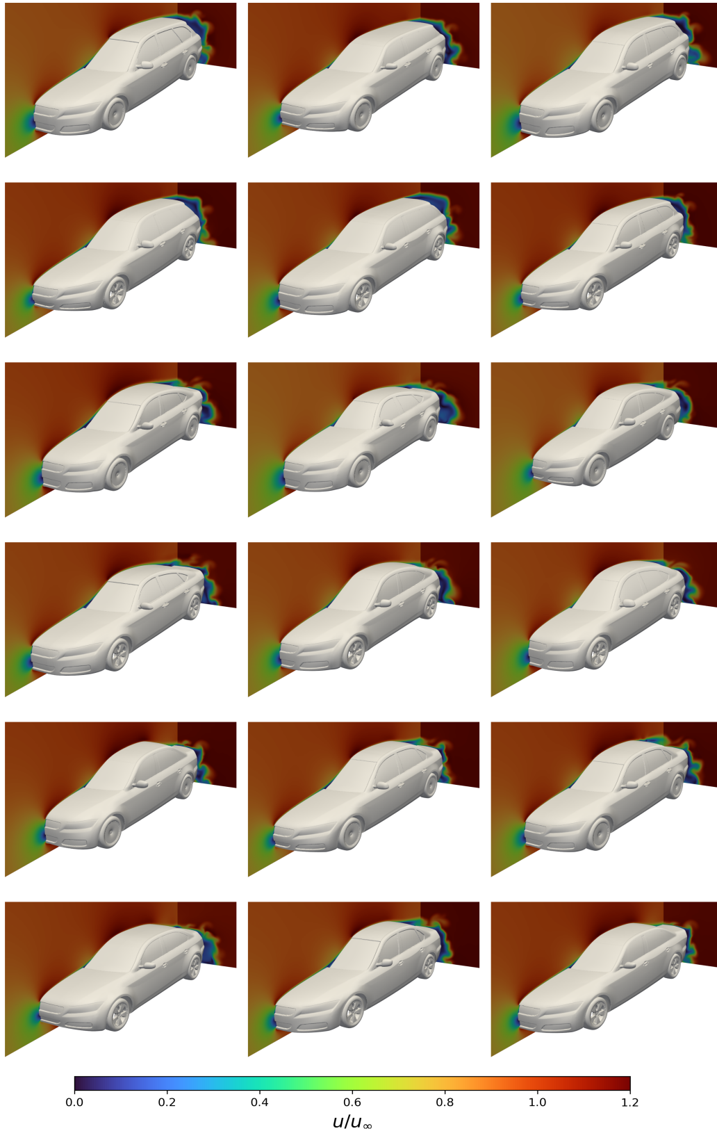
Figure 16: Visualizations of the 3D flow field around different car designs, showcasing the large variations in shape within the DrivAerNet++ dataset. The color indicates the normalized velocity u/u_\infty , with values ranging from 0 to 1.2.
