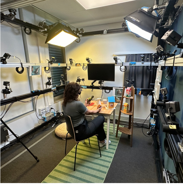
Figure 4. Motion-capture lab. The HOT3D dataset was collected using a motion-capture rig equipped with a few dozens of infrared exocentric OptiTrack cameras and light diffuser panels for illumination variability.
