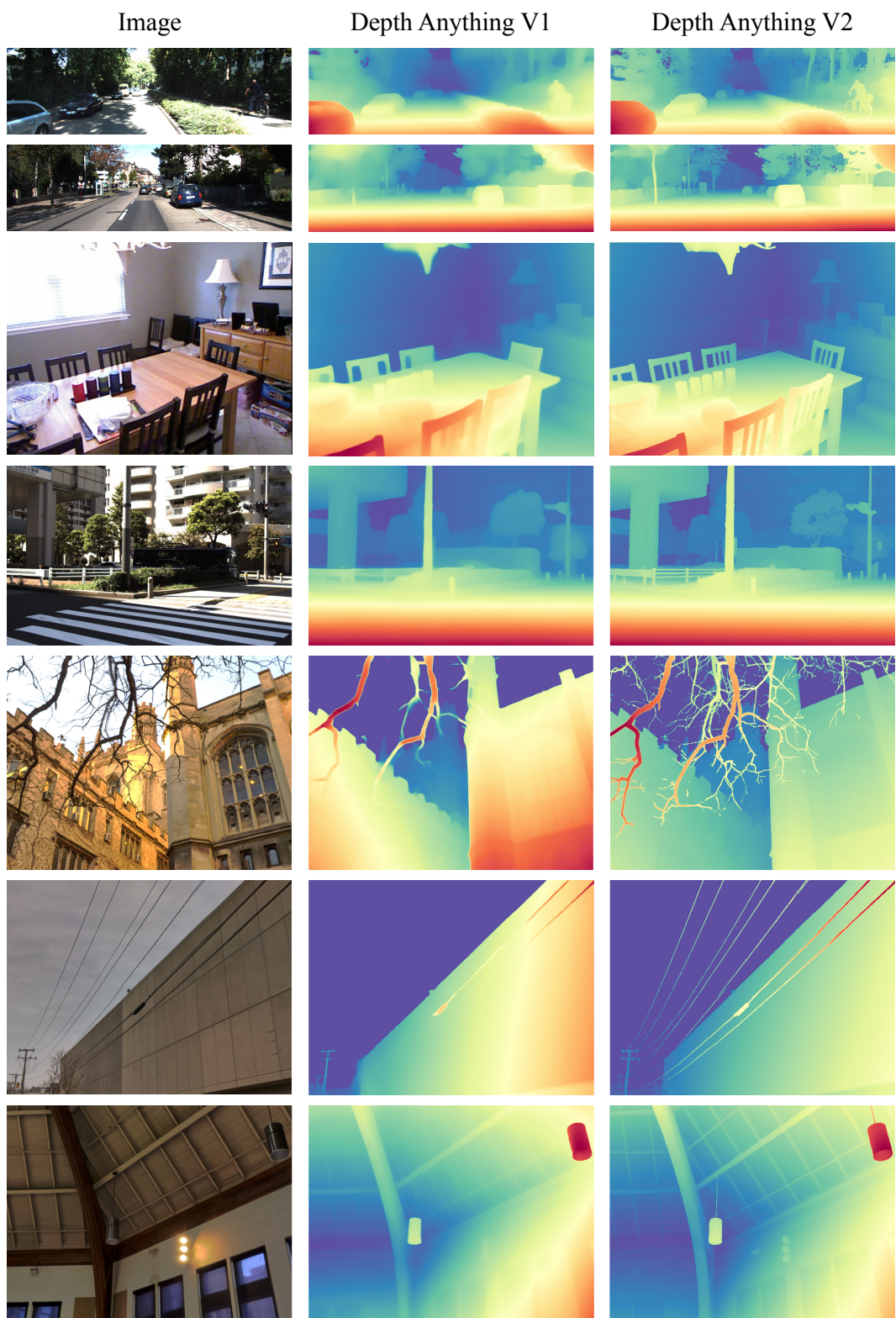
Figure 18: Qualitative results on widely adopted test benchmarks, e.g. , KITTI, NYU, and DIODE.
