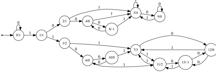
Figure 1: Automaton computing  $r_{\mathbf{t}}(n+1) - r_{\mathbf{t}}(n)$  where  $\mathbf{t}$  is the Thue–Morse sequence.
