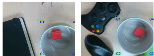
Figure 13: Two final image frames captured by the robot camera showing that D-ILVS successfully drives the robot to drop the object into the cup in different cluttered environments.
