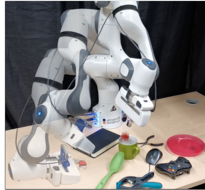
Figure 1: Our work combines off-the-shelf deep learning strategies to detect objects in the clutter, and imitation learning to realize complicated trajectories, e.g., dropping a cube into a cup on an untidy table. The large projection formulation combines the two ML components and ensures convergence to a given target.
