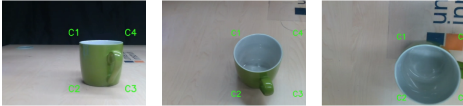
Figure 2: State-of-the-art DL-based systems like YOLO can be used to detect the features of an object of interest on raw image robustly. Examples of features are the vertices (denoted with C1, C2, C3, and C4) of the bounding box detected around the image of the object. However, such detection systems fail to capture the correct object orientation: in the three snapshots, YOLO provides very similar feature values that correspond to very different relative camera-object orientations.
