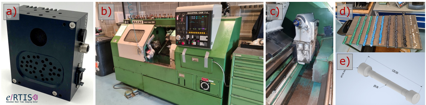
Fig. 1. Overview of the hardware setup used in this paper. Panel a) shows the eRTIS sensor, an ultrasonic array sensor with 32 microphones arranged in a pseudorandom pattern. The sensor is waterproofed using a membrane material from the Acoustic Protective Material line manufactured by W. L. Gore and Associates. Panel b) shows the CNC lathe being used, a Mazak Quickturn 10N, using Iscar GRIP 3015Y grade IC808 inserts. Panel c) shows the inside eRTIS sensor mounted in the lathe. Panel d) shows the turned materials, and e) shows the model of the piece that has been turned during this experiment.
