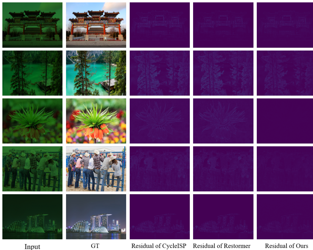
Figure 5. Visual comparison results of Demosaic for Hybridevs Camera on the evaluation dataset of MIPI-challenge 2024 track. Note that brighter means bigger error.
