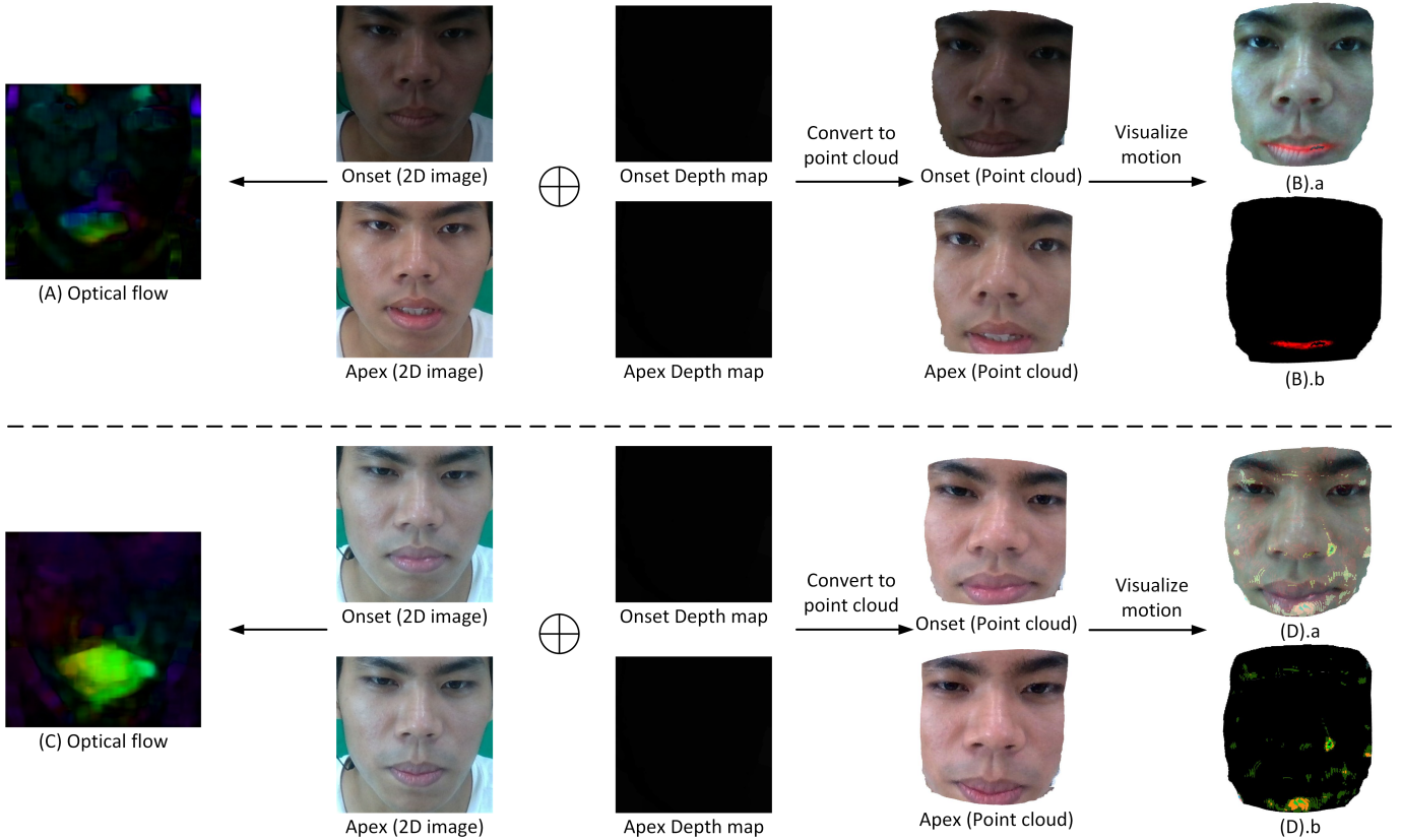
Fig. 7. Comparison of optical flow features and point cloud motion features. Where (A) and (C) are the optical flow maps of the extracted 2D image onset and apex frames. The point cloud is obtained by converting the depth information corresponding to the 2D image. (B) and (D) are the extracted point cloud motion features, where (B).a and (D).a used only to illustrate motion position; and (B).b and (D).b for further extraction of motion position.
