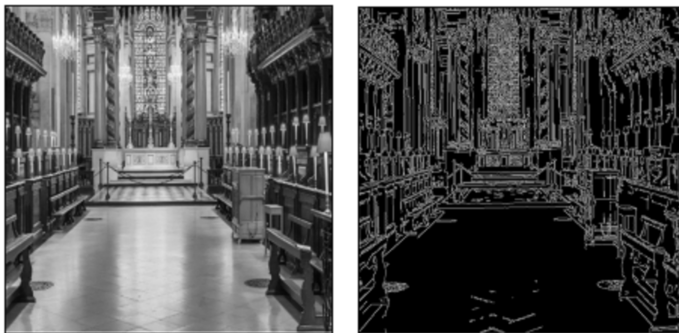
Figure 9: Left side, the original image. Right side, edges obtained by using a Canny edge detector. Taken from [2].
