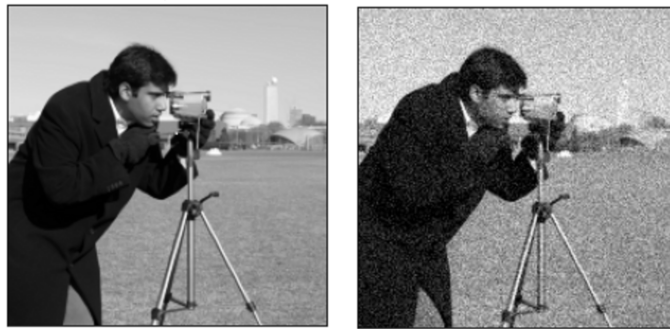
Figure 12: Left side, the original image. Right side, the image plus Gaussian noise, mean zero and variance 0.05. Taken from [2].
