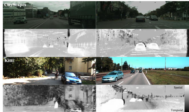
Fig. 12. Temporal-Spatial Uncertainty Fusion: White represents higher reliability in spatial reprojection, while black represents higher reliability in temporal reprojection, as shown in the legend in the bottom right corner. We can observe that non-rigid moving objects in the image tend to reproject more in space (white). Meanwhile, occluded areas and distant regions tend to reproject more in the temporal sequence (black), and the remaining areas show no significant tendency (gray).
