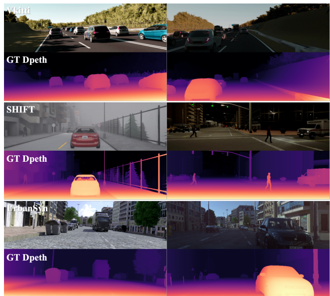
Fig. 13. The synthetic datasets: In vKitti2, depth cannot penetrate transparent entities such as glass windows, whereas in the SHIFT dataset, depth can penetrate transparent entities. SHIFT and UrbanSyn includes simulated pedestrians. And UrbanSyn is the synthetic dataset that most closely resembles real world.
