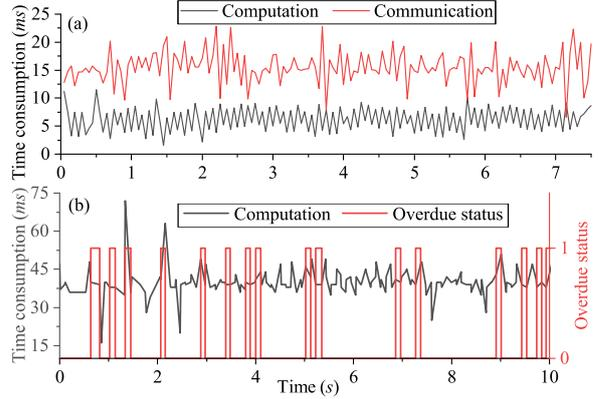
Figure 10: Comparison of the time consumption of real-time control when the CPG is calculated at (a): edge server, (b): robot’s onboard controller.
