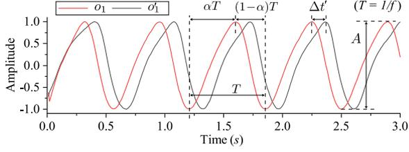
Figure 2: The non-harmonic oscillator response with varying frequencies. In this example, the initial state is randomized, and  $[A, f, \alpha, \tau, k, \epsilon, \Delta t'] = [1, 1.33, 0.75, 1, 1000, 5, 0.25]$ .
