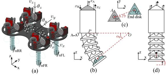
Figure 1: Overview of the soft robot and its Tendon-driven Soft Actuator (TSA): (a) Rendered robot with key states. (b) Structure of TSA: rigid upper thigh and bendable lower section with  $\alpha_b$ . (c) Top view of bent TSA with  $\alpha_r$ . (d) TSA compression via equal tendon pull with  $z_1$ .
