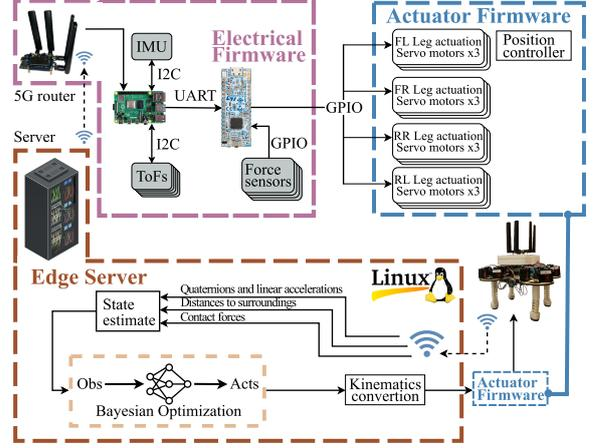
Figure 3: Control system architecture. The actuator and electrical firmware are physically integrated into the robot. The unidirectional arrows surrounding radio waves denote the transmission and reception of messages between soft robots and the edge server.
