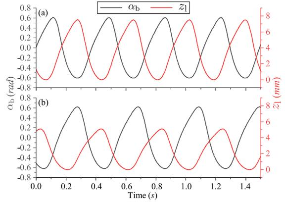
Figure 9: Comparison of behaviors of optimized oscillators. (a): Simulation platform, (b): Physical testing platform.
