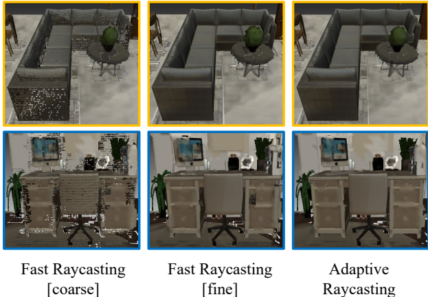
Figure D. Adaptive raycasting. We show the reconstructed map of MAP-ADAPT-SG with adaptive raycasting and fast raycasting [33] in the coarse and fine resolutions.
