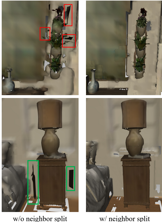
Figure E. Neighbor splitting. We show the reconstructed map of MAP-ADAPT-SG with and without neighbor splitting. Ghost meshes are highlighted in the color boxes.
