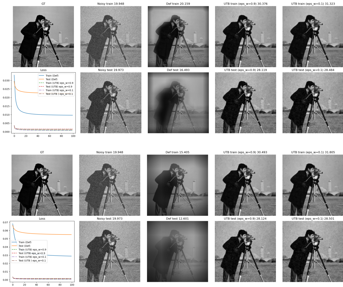
Figure 7: Results of learnt deformable and our metric UTB convolutions with \sigma_n = 0.1 and k = 51, 121 from top to bottom.
