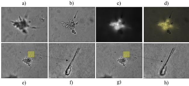
Figure 3. Visualization of a) Out-of-focus slice ( $Z=13$ ); b) Partially in-focus slice ( $Z=6$ ); c) and d) In-focus detection map of image b) and its overlay image; e) and f): Output images of SBS-Stacking; g) and h): Output images of normal Focus-Stack.
