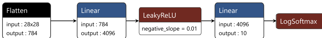
Figure 1: Neural architecture used in this work for MNIST and Fashion-MNIST classification task.
