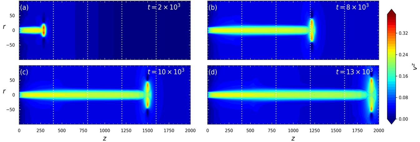
**Figure 11.** Contours of  $v^z$  for an electron-proton jet.
