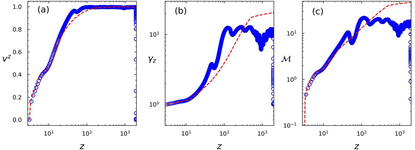
**Figure 3.** Variation of  $v^z$ ,  $\gamma_z$ , and relativistic Mach number  $\mathcal{M}$  is plotted in panel (a) to (c). The dashed red line represents the solution for a steady-state jet, and blue open circles correspond to the variables along the jet spine of the 2D simulation.
