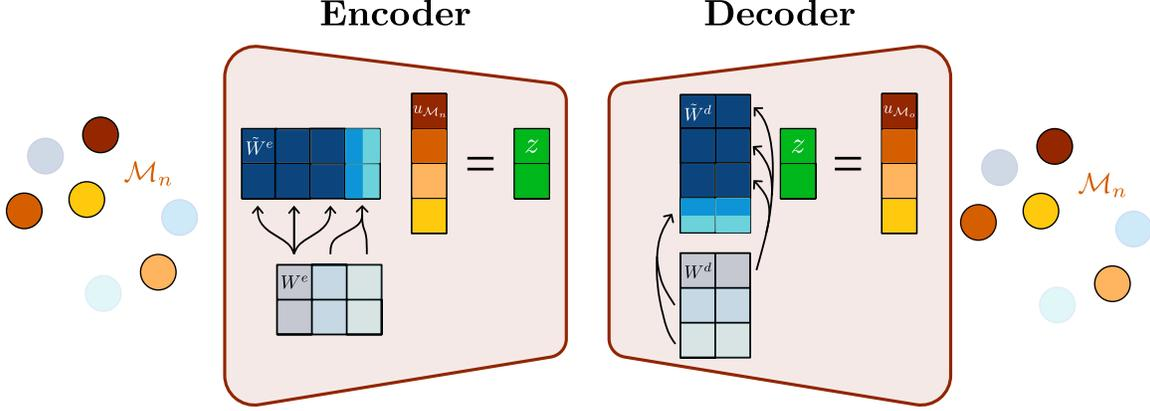
FIGURE 5. GFN approach to transform weights between meshes. Light blue shades denote the original mesh with its associated  $\mathbf{W}^e$  and  $\mathbf{W}^d$ . The arrows depict how the new weight matrices (in darker blue shades)  $\tilde{\mathbf{W}}^e$  and  $\tilde{\mathbf{W}}^d$  can be created from the original weights and used for prediction on the new mesh.
