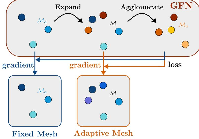
FIGURE 9. Training with fixed or adaptive mesh methods when given a starting mesh  $\mathcal{M}_o$  and new mesh  $\mathcal{M}_n$ . The fixed mesh approach updates the original mesh weights, whilst the adaptive mesh approach updates weights on a new mesh  $\mathcal{M}$ , created from information from both meshes.
