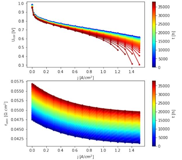
Figure 4: Simulated polarization curves (top) and ohmic resistance (bottom) as functions of current density every 500 hours.
