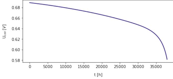
Figure 5: Simulated voltage over time, with current density fixed at  $1A/cm^2$ .
