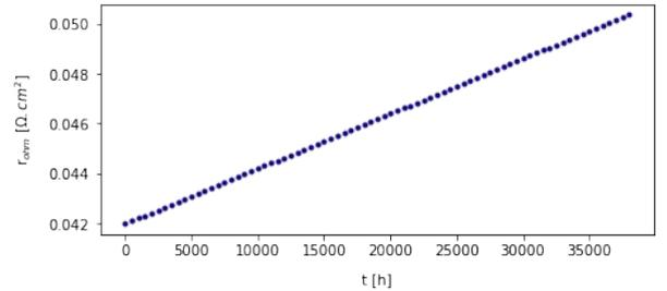
Figure 8: Temporal evolution of  $r_{ohm}$  at  $1A/cm^2$ .
