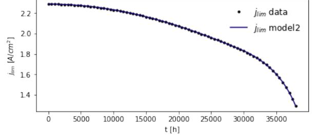
Figure 11: Fitted curves of  $j_{lim}$  with model2 (Equation 11).
