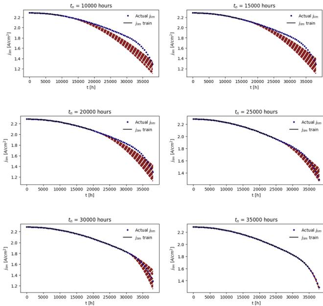
Figure 13: Simulation of 500  $j_{lim}$  curves for different learning durations. The red curves represent the simulated scenarios.
