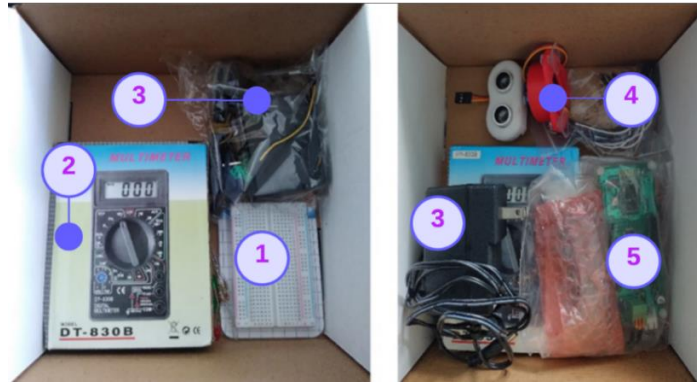
Figure 2. Example of the hardware materials sent to the students. 1. Protoboard, 2. Multimeter, 3. 12V DC adapter, 4. Robot in 3-D printing, 5. Compatible Arduino development board and LCD.
