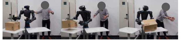
Fig. 1. Operating a humanoid with the developed controller. Our teleoperation controller does not require paired data sets or common pre-specifications for its learning process to achieve human-to-humanoid motion retargeting.
