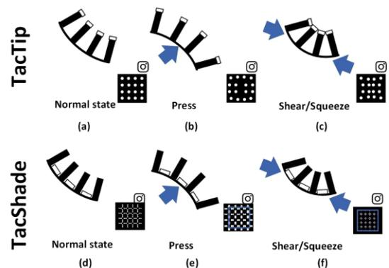
**Fig.2** Design-concept of TacShade and its compare with Tactip. (a) to (c) show the state of TacTip's pins and markers in normal state, press and shear/squeeze, and (d) to (f) show the state of the TacShade.
