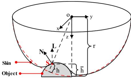
**Fig.5** Simplified contact deformation model of the TacTip (include TacShade). The red dotted line indicates the skin without contact. The degree of deformation at point S on the skin caused by contact with the object is represented by  $h$ .
