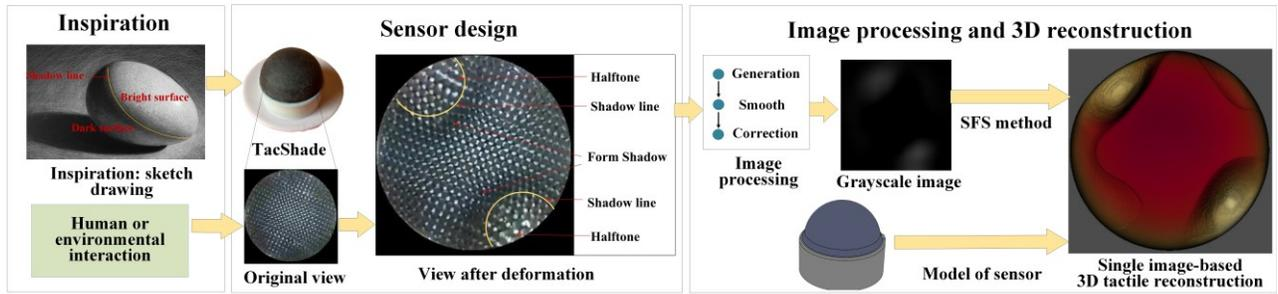
**Fig.1** Diagram of TacShade for single image-based 3D tactile reconstruction. Under the inspiration of sketch drawing, the research of TacShade consisted of two aspects: sensor design in hardware and image processing in software to achieve final tactile 3D reconstruction effect.
