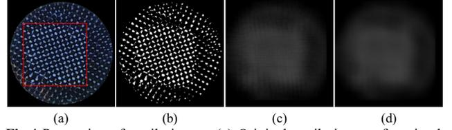
**Fig.4** Processing of tactile image: (a) Original tactile image after circular mask filtering, and the red box highlights the skin deformation area of the rectangular contact head; (b) Binary tactile image; (c) and (d) Greyscale tactile image before and after TVD filtering.
