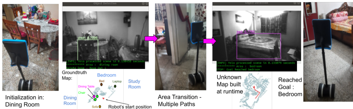
Fig. 18: Real life example of ‘AreaGoal’ task. Starting at dining room, the robot needs to navigate to bedroom.
