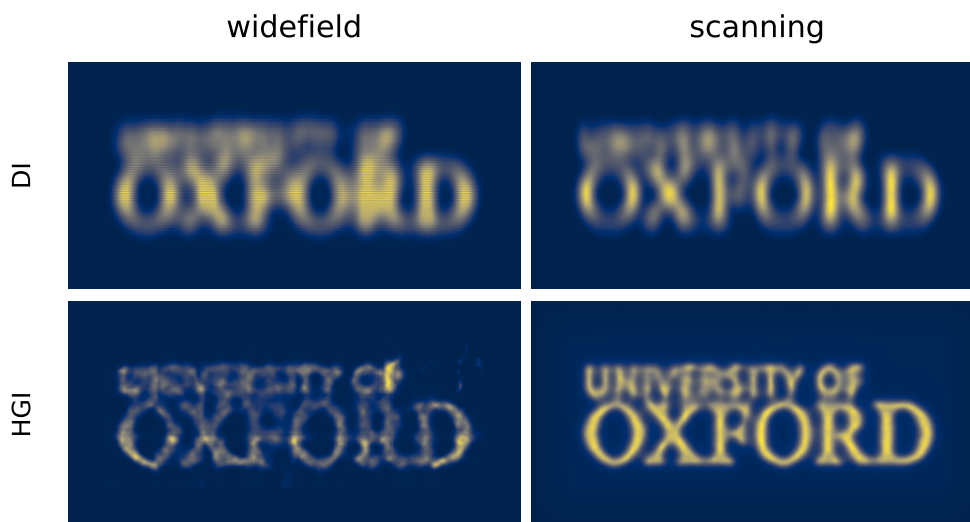
Fig. 4. Imaging the Oxford University logo using DI and HGI under widefield and focused scanning illumination.
