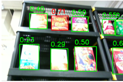
Figure 8: A sample product detection result that was robust to blurring and overexposure with the help of data association.
