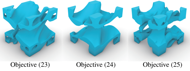
Fig. 14 Comparisons of different objective functions. The target tensor is [0.3, 0.2, 0.1, 0.05, 0.05, 0.05] . The resulting thermal conductivity tensors from left to right are [0.293, 0.198, 0.097, 0.043, 0.050, 0.046] , [0.286, 0.190, 0.095, 0.046, 0.048, 0.039] , [0.274, 0.198, 0.098, 0.050, 0.048, 0.048] .
