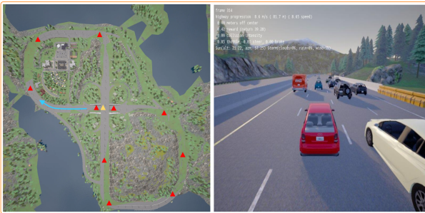
Fig. 7. Left: An aerial view of the CARLA-Town04 map, in which triangles represent some of the officially provided spawn/start points, and the blue arrow represents the driving direction; Right: A live photo, in which the red vehicle in the center is the trained vehicle agent and the others are NPC vehicles.
