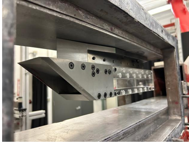
Fig. 2 Inlet model, attached isolator, and acrylic wall configuration of the NCSU model
