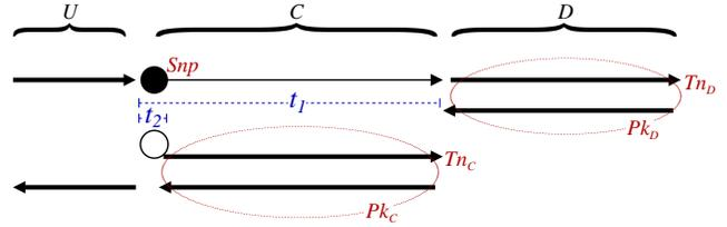
Figure 2: Sketch of execution for the adjoint of the same code than in Fig. 1, this time checkpointing code part  $C$ . Time goes top-down, and inside each line time follows the arrows direction. The thin arrow to the right stands for the extra execution of the primal  $C$ , and the black and white bullets stand for respectively the writing and reading of the *snapshot*, i.e. a set of variables sufficient for identical duplicate execution of  $C$ .
