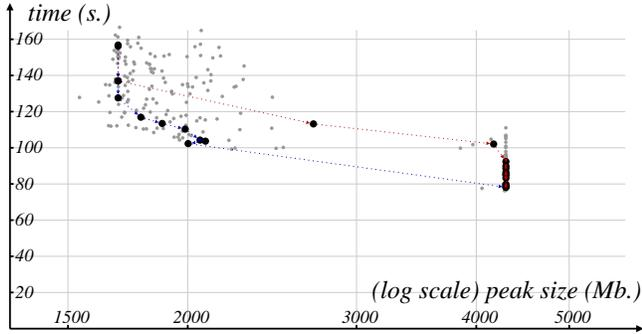
Figure 5: Tuning the adjoint of `tutorial_global_oce_biogeo` by profiling. Each checkpointing configuration is shown as a dot whose coordinates are peak stack size and run time of the adjoint. The red and blue lines show the evolution of performance guided by profiling, respectively with a “run-time gain first” strategy, and a “careful on memory” strategy. Gray dots show the performance of 250 random checkpointing configurations.
