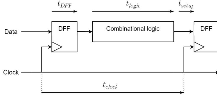
Fig. 3. Timing constraints in a digital system
