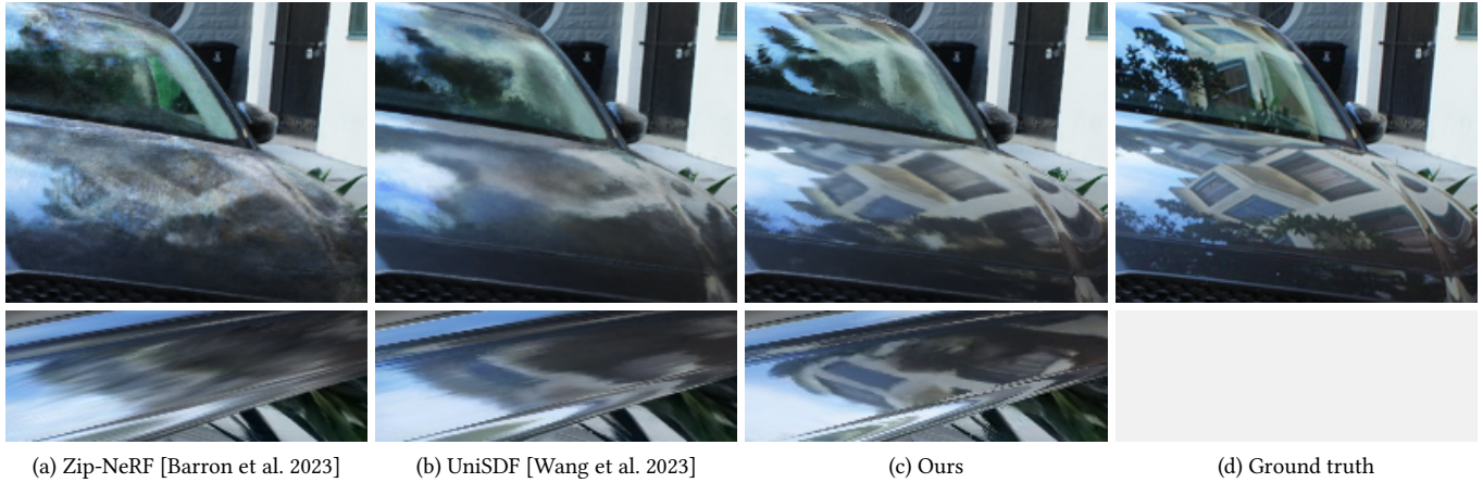
Fig. 1. Our method, NeRF-Casting, recovers and renders scenes with higher-quality reflections than prior work. Here we show cropped renderings and a ground-truth image for a scene in our dataset (top), as well as a slice from a video rendering along a smooth camera path (one horizontal row of pixels stacked vertically across multiple video frames) to emphasize the continuity of high-frequency reflected content in our result (bottom). Please see the videos provided in the supplemental webpage to observe the accurate motion of our rendered reflections.
