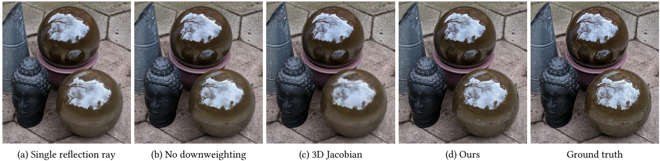
Fig. 5. Ablation of our reflection anti-aliasing components. Using (a) a single reflection ray instead of five, (b) not downweighting reflection features, or (c) using Zip-NeRF’s 3D Jacobian instead of restricting it to the 2D directional Jacobian, all result in inaccurate reflections. Even for low-roughness objects such as the shiny spheres shown here, aliasing in the reflections during optimization prevents the model from accurately reconstructing both the reflective surface geometry as well as the reflected content.
