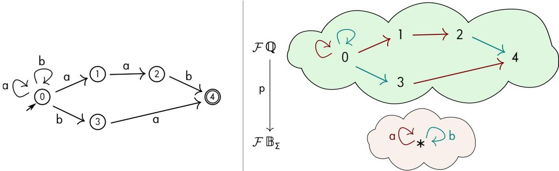
Figure 4: Left: an NFA represented with a traditional state-diagram. Right: the bare NFA as a finitary ULF functor  $p : \mathcal{F} \mathcal{Q} \rightarrow \mathcal{F} \mathbb{B}_\Sigma$ . (We do not label the generators of  $\mathcal{F} \mathcal{Q}$  or indicate composite arrows, and we use colors to indicate the images of the generators in  $\mathcal{F} \mathbb{B}_\Sigma$ .)
