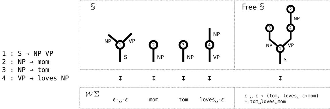
Figure 2: Example of a context-free grammar represented by a functor  $\mathcal{F} \mathbb{S} \rightarrow \mathcal{W}\Sigma$ , where we have indicated the action of the functor on the generators as well as the induced action on a closed derivation tree.
