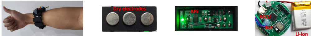
Figure 11: In-house developed sEMG acquisition system: from left to right are the acquisition system, dry electrodes, AFE, MCU with BLE 5.2 module, respectively.
