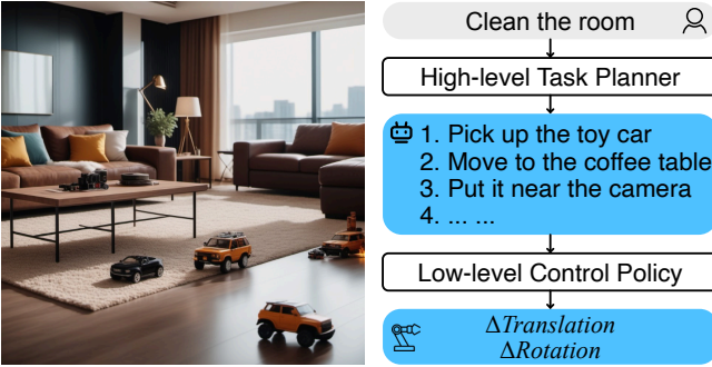
Figure 3: Illustration of a hierarchical robot policy comprising a high-level task planner and a low-level control policy. The high-level task planner generates a plan based on the user instruction, which is then executed step by step by the low-level control policy.
