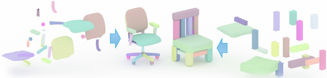
Figure 10: Assembly of semantic parts. Given parts in random positions (left and right), the network assembles them into complete shapes (middle). We solve this part-assembly problem via preserving the attributes of part shapes and scales and only generating the attribute of part positions.
