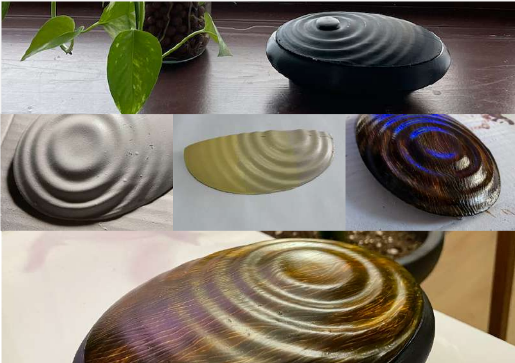
Figure 5.11 Final Painting Process a) 3D Prints, b) Primed, c) Sanded, d) Aged, e) Final
