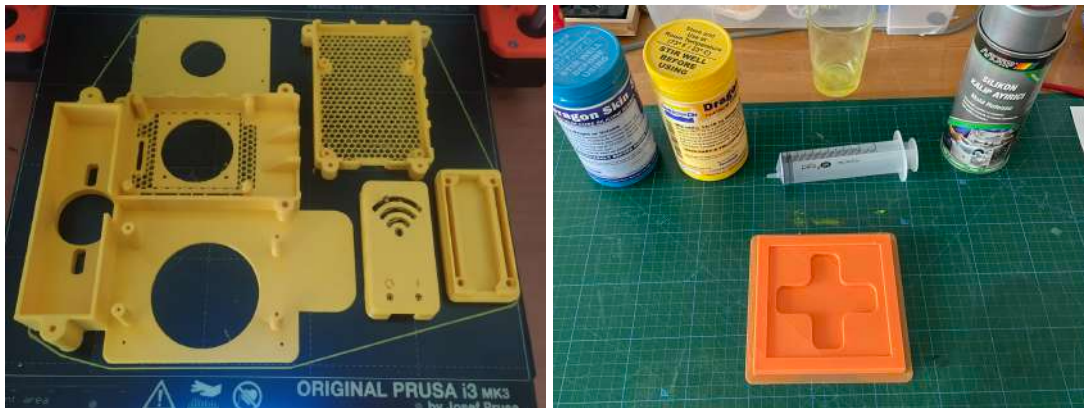
Figure 7.16 a) 3D Printed casing for the electronics, b) The mold for plus-shaped surface
