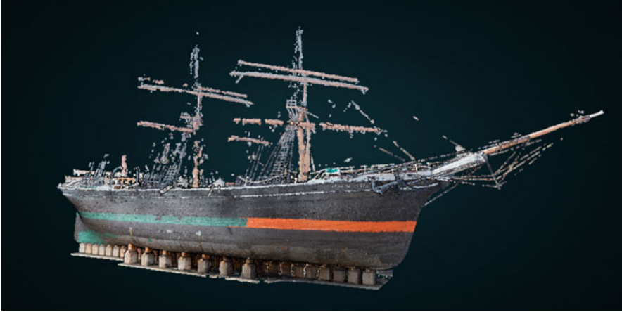
Fig. 1 Point cloud representation of the Star of India obtained through photogrammetry (courtesy of Scott McAvoy on Open Heritage 3D)
