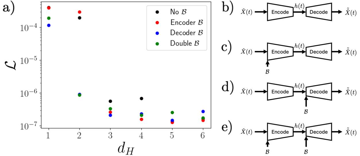
FIG. 6. a) Loss over the testing data for each autoencoder architecture as a function of latent dimension. Block diagrams for the autoencoder neural network architectures (b) “No  $\mathcal{B}$ ”, (c) “Encoder  $\mathcal{B}$ ”, (d) “Decoder  $\mathcal{B}$ ”, and (e) “Double  $\mathcal{B}$ ”.
