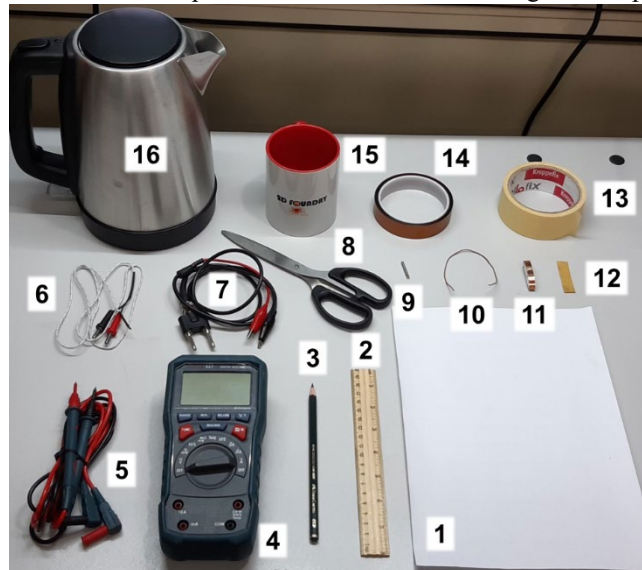
Figure 1. Materials. 1 Paper sheet. 2 Ruler. 3 Pencil. 4 Multimeter. 5 Probes. 6 Thermocouple. 7 Crocodile cable. 8 Scissors. 9 Magnets. 10 Wire. 11 Copper tape. 12 Double sided tape. 13 Masking tape. 14 Kapton tape. 15 Mug. 16 Kettle.
