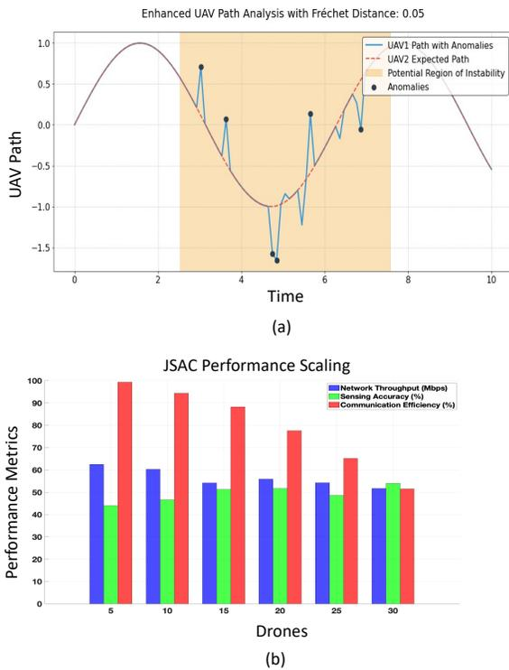
Fig. 4. (a) A comparison of UAV trajectories in ISAC analysis by revealing sensing anomalies in UAV1’s path where the shaded region indicates a potential zone of instability; (b) The scaling impact of ISAC performance in UAV networks with increasing drone numbers.
