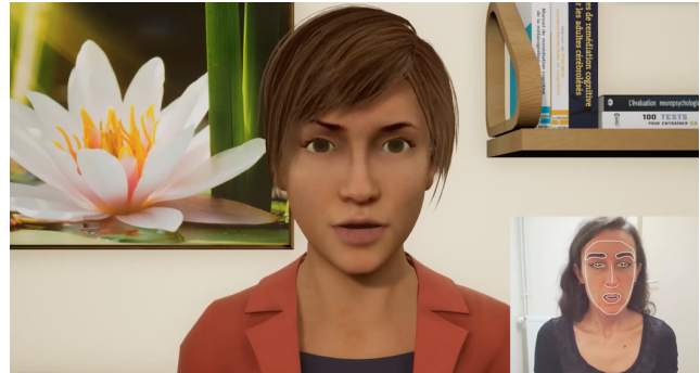
Fig. 1. Head movements, gaze, speech, and articulation of a remote operator were captured in real-time to drive a virtual assistant as a Wizard-of-Oz [6].
