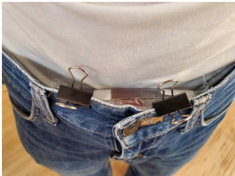
Fig. 2: Attachment of abdominal movement measurement device
